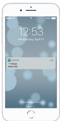
An alert notification is delivered directly from the physiologic monitor to the primary nurse
